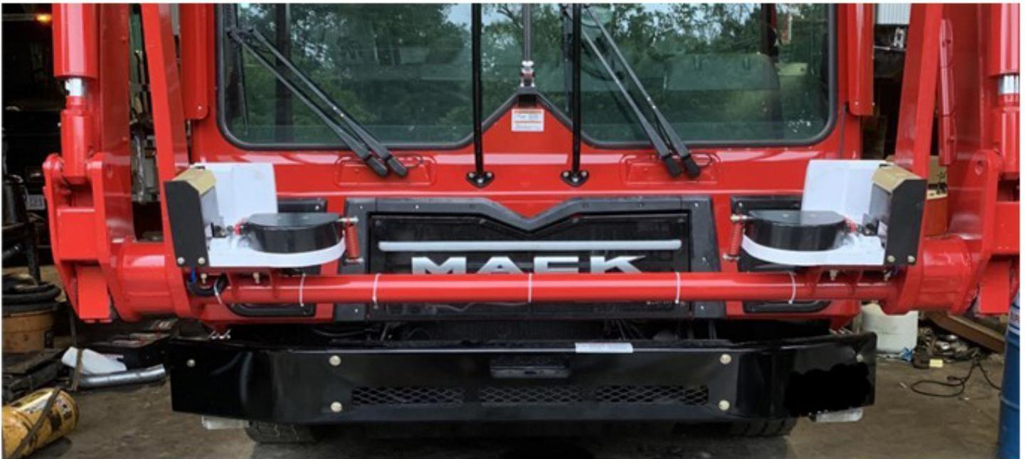
It's only been over the last 5 years that the use of front-load trucks to service the all rear-load dumpster and mixed RF / FL routes has taken off. This has been made possible by the costly introduction of welding [side] fork-pockets on existing RL dumpsters... or by the new, alternative method of installing an aftermarket pair of Johnny Jaws on a front-load truck.
